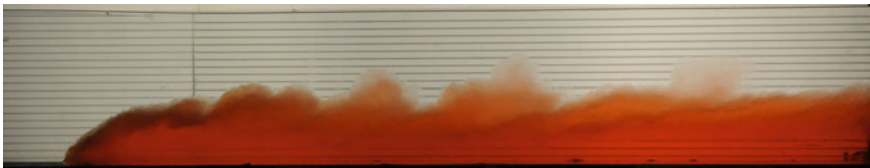
Fig. 12 Visualization of a gravity current. The current is dyed with food colouring and viewed against a translucent lined sheet. Courtesy of Hughes and Linden (2016)
